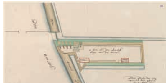
Outpost on the Amsteldijk opposite the one near the Omval. A row of piles with lockable navigation openings blocked the river Amstel. The hole in the dike was resealed in 1673
