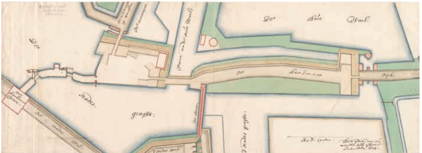
5. Cornelis Koel, Reinforcement in front of the Haarlemmerpoort in the Disaster Year. A ravelin encompassed the Haarlemmerweg and the barge canal. An elongated fortification along the Spaarndammerdijk guarded the locks in the dike and the brick dam separating the city moat from the IJ. Map from 1674 (Stadsarchief Amsterdam)
