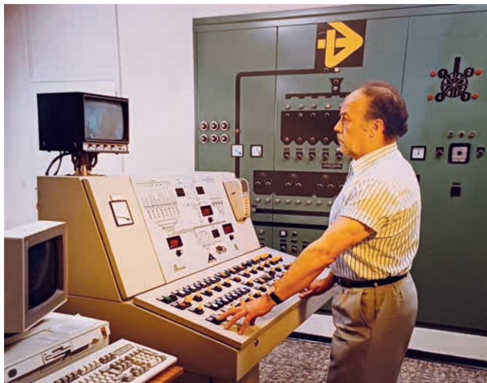
9. Growing scientific precision in the production of concrete mixes: note the graphical representation of various aggregate silos on the control panel. Research at Inter-Beton contributed to the standardization of ready-mixed concrete and the BENOR/SECO label (Belgian State Archives, CBR Fund, 3519)
