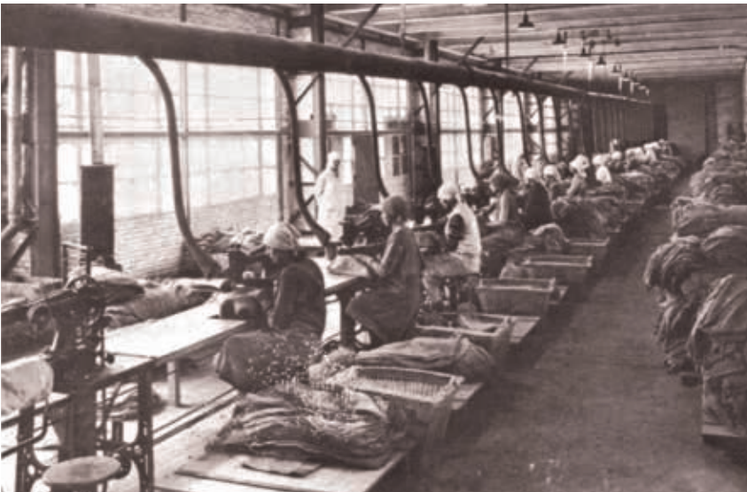
5. CBR factory in Lot, where cement bags were for a long time sewn from jute. Right: paper bags did not predominate until after the Second World War, while cement distribution remained highly labour-intensive for a long time (CBR Echos (1981) 85, 9; VCN, Cement , 1970, 46)
