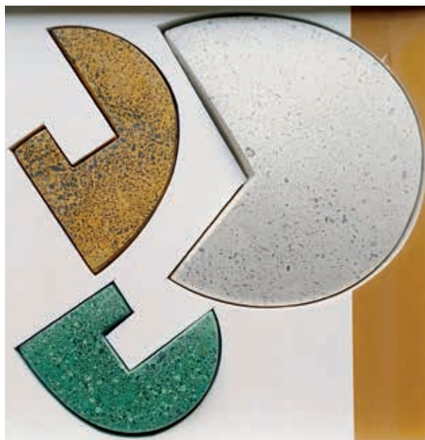
15. Overview of various Inter-Beton mixes specially developed for every conceivable use. Samples of MAR-mix in all possible shapes and colours (Sint-Pieters-Leeuw concrete plant archive, not inventoried)
